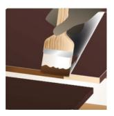
After cutting the panel, apply an acrylic-based water-resistant paint to the edges to prevent swelling caused moisture.
