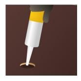
Seal all holes drilled during installation with silicone adhesive to prevent swelling from moisture.
