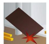
When removing the the shuttering, ensure plywood panels are neither dropped nor dragged on the ground.
